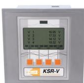
Multi-function capacitor protecting relay for unbalance supervision of 3-phase capacitor banks via 3 x 2-pole voltage transformers secondary connections open delta (voltage unbalance supervision)
