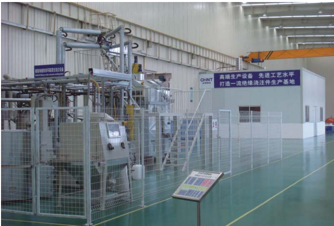
Compact Vacuum Casting Equipment
