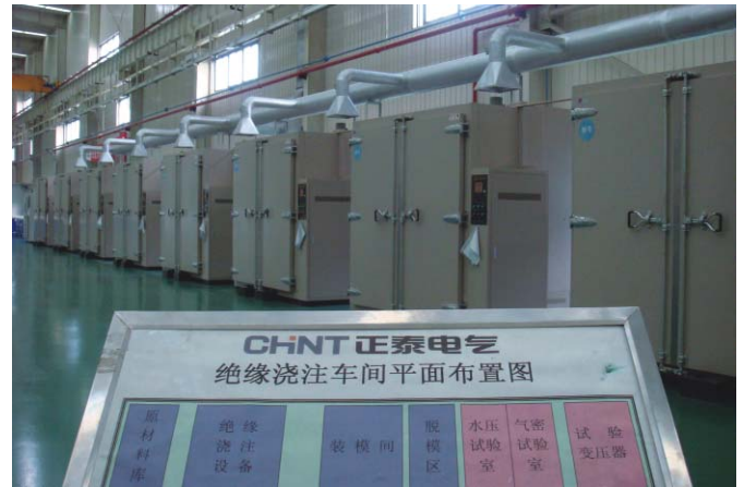
Curing furnace for manufacturing of basin-type insulator
