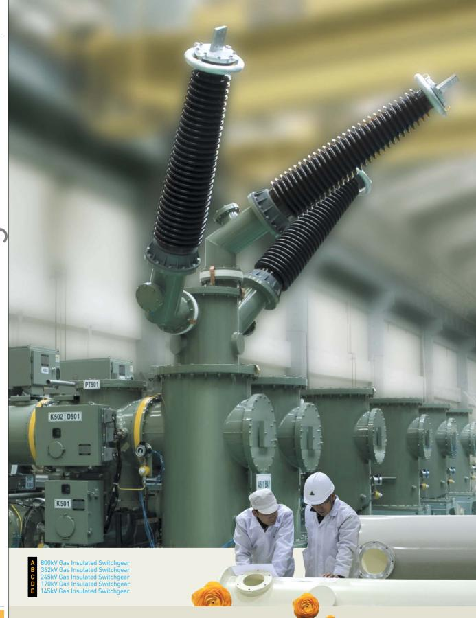
he SF<sub>6</sub> Gas Insulated Switchgear(GIS) contains the major equipment used in a substation such as gas circuit breaker, disconnecting switch, earthing switch, voltage transformer, current transformer, lightning arrester, etc. in a grounded metallic enclosure. The switchgear is filled with SF6 gas, which has the best insulation and arc-quenching capabilities.
