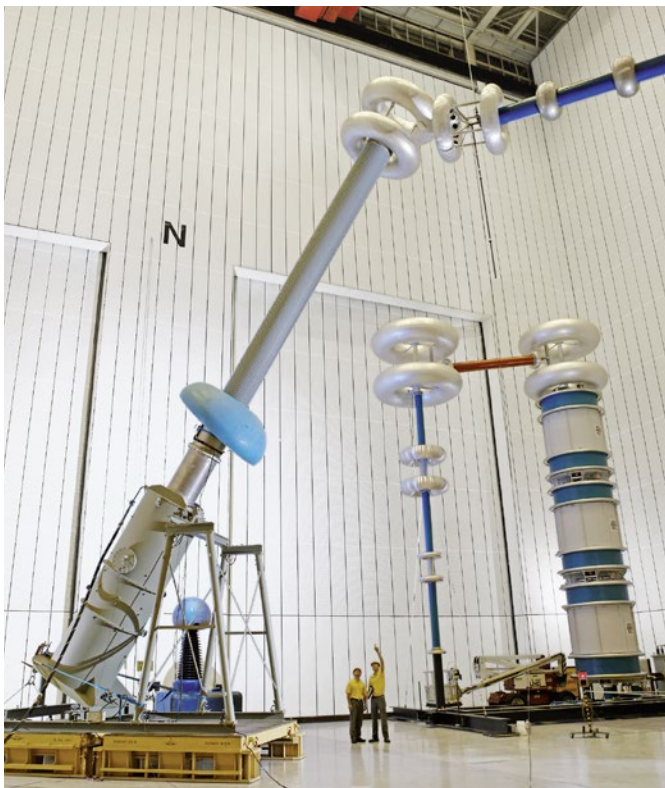
Fig. 4.8-5: Transformer bushing – 800 kV UHVDC – project Yunnan-Guangdong, China
