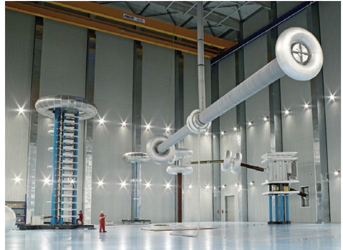
Fig. 4.8-8: Wall bushing – 800 kV HVDC – project Yunnan-Guangdong, China
