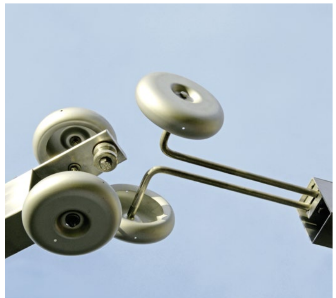
Fig. 4.2-2: Block and finger contact system
