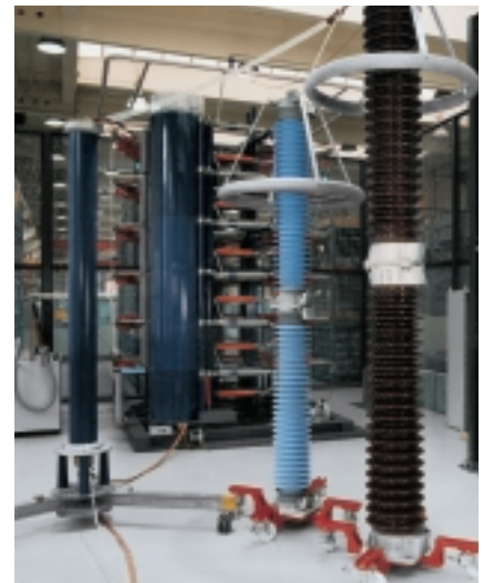
Fig. 34: Measurement of residual voltage on porcelain-housed (foreground) and polymer-housed (background) arresters
