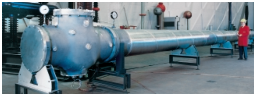
Fig. 61: Siemens lab prototype for dielectric tests
