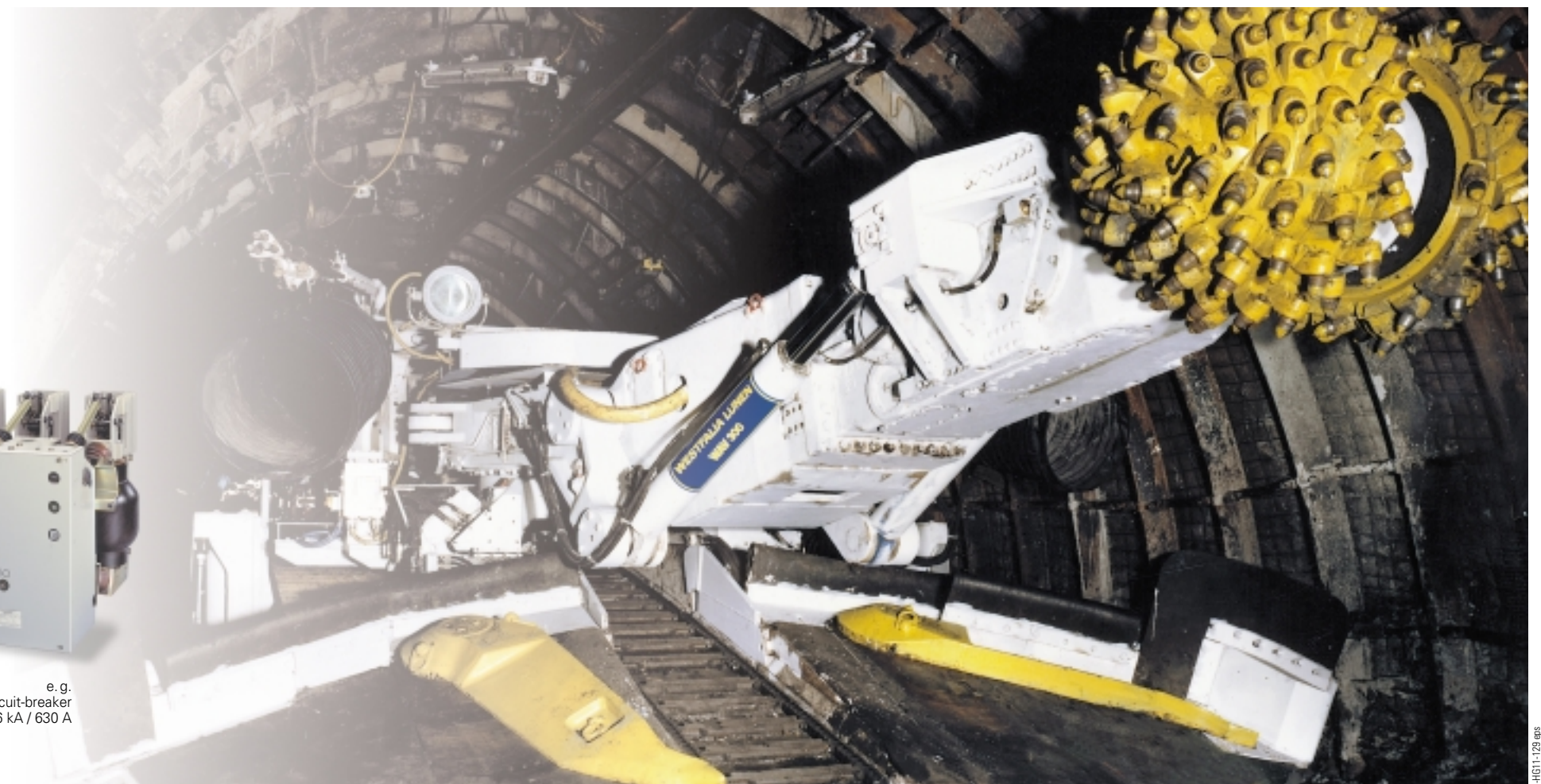
Mobile selective-cut road driving machine for underground mining type WAW 300 (photo Westfalia Lünen)
