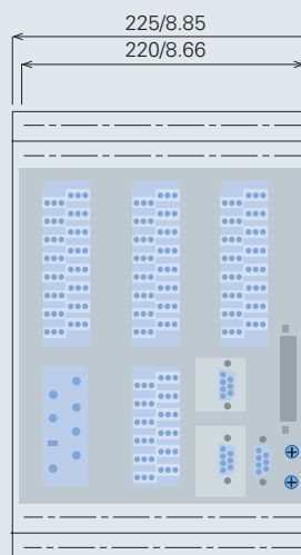
Fig. 77: 7SJ63, 1/2 surface mounting case (only with detached panel, see Fig. 42, page 6/21)
