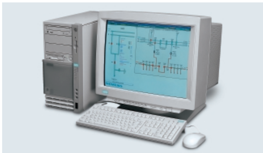
Fig. 136: Digital substation control, operator desk. Control of a 400 kV substation (double control unit)
