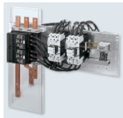
Fig. 269: 4RY56 Capacitor module 100 kvar, switchable as 2 x 50 kvar module for cable connection
