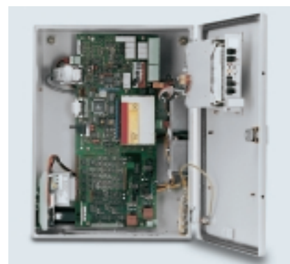
Fig. 171: 6MB5530-1 remote terminal unit (RTC) with cable-shield communication
