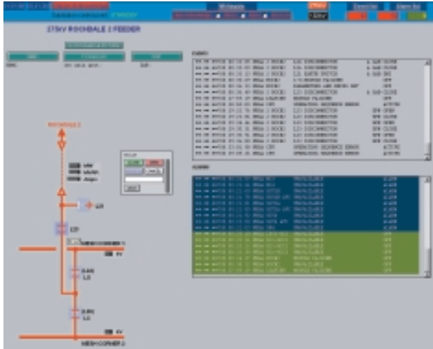
Fig. 153: SINAUT LSA substation control, example: overview picture
