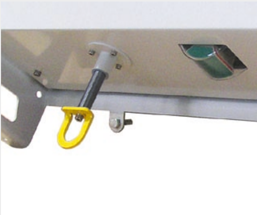
Lockout handle – pulled (open position)
