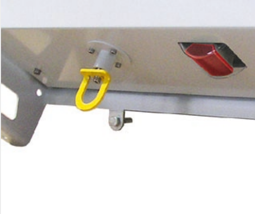
Lockout handle – pushed in (operational position)
