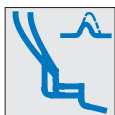
Circuit-breaker for system and generator protection, ETU20, LSI function for time-based discrimination (S function: t_{sd} = 1.5 to 10 \times I_R , t_{sd} = 0 to 0.5 s)
