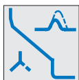
Circuit-breakers for motor/generator protection, ETU10M, LI function with permanently set time-lag class t_R = 10 , with phase failure sensitivity
