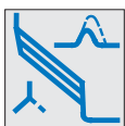
Circuit-breakers for motor protection, ETU30M, LI function with adjustable time-lag class t_R (10A, 10, 15, 20, 30), with phase failure sensitivity
