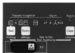
Indication on electronic trip unit version N
