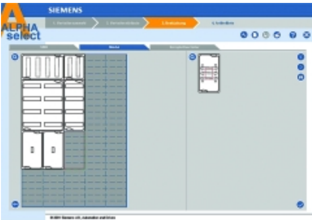
ALPHA SELECT construction of the distribution boards
