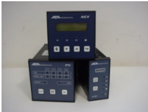
Figure 20 Thermocontroller and fans control relay
