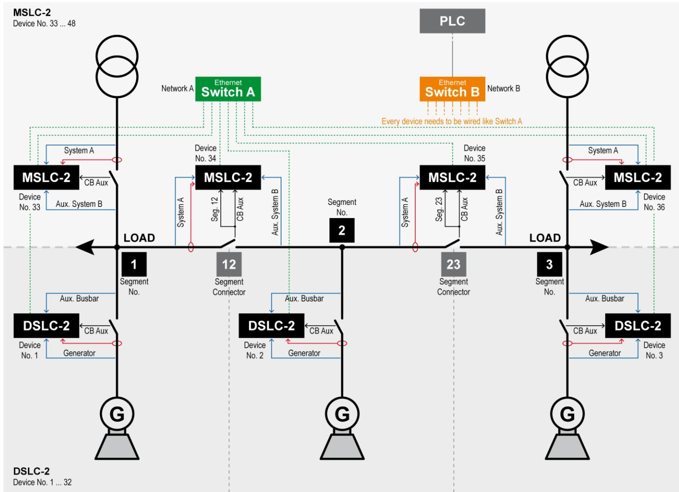
Configuration of a typical application using DSCL-2 und MSLC-2 devices in combination
